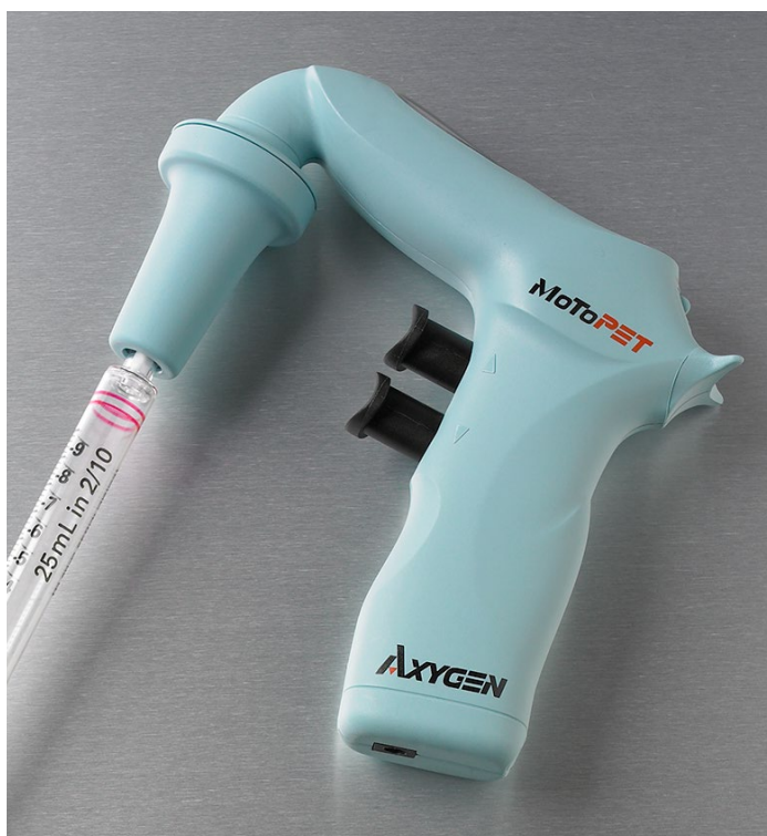
Pressure sensitive trigger buttons control rate of aspiration or dispensing.
