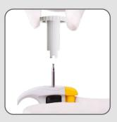
Insert the calibration key into the calibration knob. The calibration key is supplied with the pipettor.
