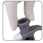
A calibration key is provided with each pipettor to enable user calibration
