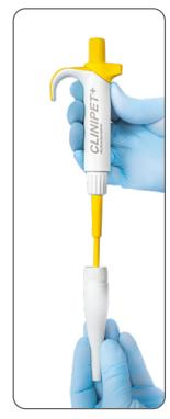
Easy removable tip ejector enables easy work with narrow tubes.
