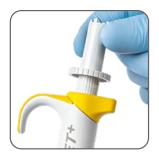
Recalibration system allows for quick and accurate pipettor calibration
